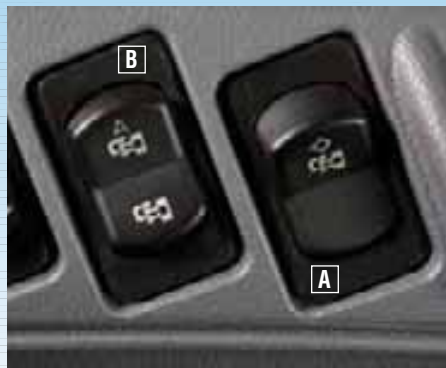
These switches on the right-hand console are used to alert the system that you are ready to record (A) or play back (B) a sequence of actions. Then, press the “step” button on the multi function controller (C) to actually activate the recording or playback.
