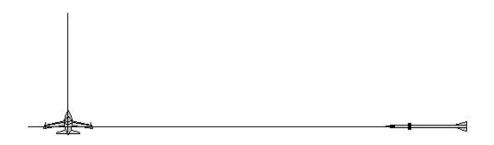
The missile's guidance system keeps it pointing at the jet at all times.
