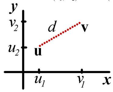
$$d^2 = (v_1 - u_1)^2 + (v_2 - u_2)^2$$
