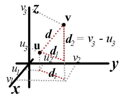
$$d_1^2 = (v_1 - u_1)^2 + (v_2 - u_2)^2$$
