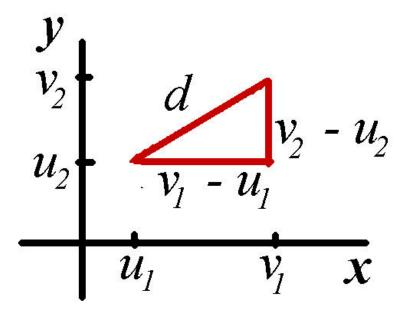
$$d = \sqrt{(v_1 - u_1)^2 + (v_2 - u_2)^2}$$
