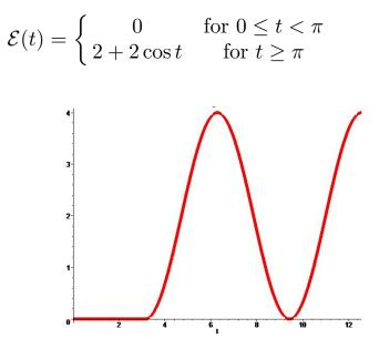
Notice that  $\mathcal{E}(t) = (2+2\cos t)\mathcal{U}(t-\pi)$ . Let's solve the differential equation and obtain a formula for y(t) (how charge on the capacitor varies with time).
