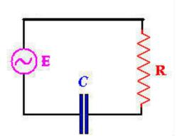
On the capacitor, the ratio of the charge to the voltage drop remains constant:
